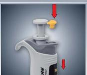
Insert the calibration key into the ejector orifice. Turn the key so as the volume indicated by the counter is equal to the average calculated volume.
