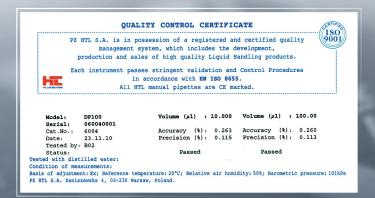
Each HTL pipette is supplied with an individual QC certificate, attesting the strict factory control and excellent performance values obtained. Conformity to ISO 8655 and IVD 98/79/EC Directives. The production standards set by the manufacturing quality management systems – certified to ISO 9001/2000.
